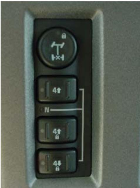
Your H2's full-time four-wheel-drive system can be operated in five different modes, depending on road conditions:
