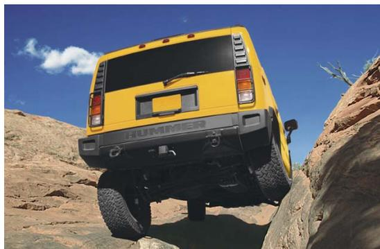
4-Low Lock with rear differential locked mode should be used only when you need maximum traction in low-speed situations, such as when climbing over large rocks or up long, steep grades.
