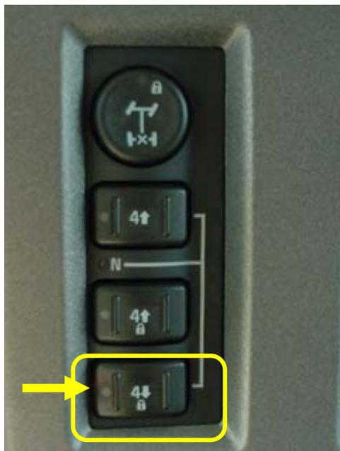
To shift to 4-Low Lock, the engine on your H2 must be running and the vehicle must be stopped or traveling at less than two miles per hour...or 3.2 kilometers per hour...with the transmission in Neutral, press and release the 4-Low button.
