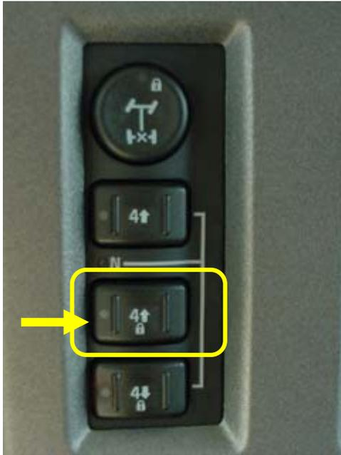
To shift into the 4-HI Lock mode, be sure your H2 is traveling at less than 40 mph...or 64 kilometers per hour...and press and release the 4-High Lock button.
