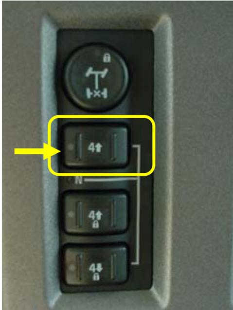
To shift into the 4-High mode, be sure your H2 is traveling at less than 40 mph...or 64 kilometers per hour...and press and release the 4-High button.
